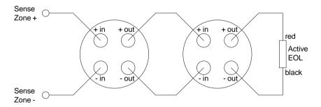
The panel is supplied with 3k3 end of line resistors as standard. Active end of line units are available separately.
