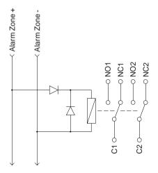
A relay may be connected anywhere on the alarm zone wiring provided that two diodes (1N4001 or equivalent) are fitted as shown in the diagram. The end of line resistor is not shown, but must be connected at the end of the alarm zone wiring. The relay must have a 24V DC coil.
