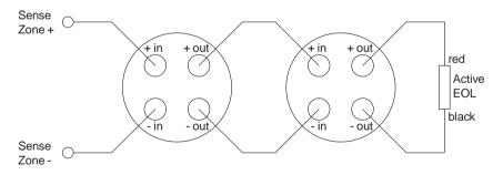
The panel is supplied with 3k3 end of line resistors as standard. Active end of line units are available separately.
