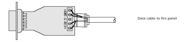
The data cable should be secured to the converter using the cable clamp and routed such that it is not likely to be stressed.
