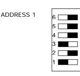
Shows switch actuator in the ON position. For Address 32 all switches must be off.
