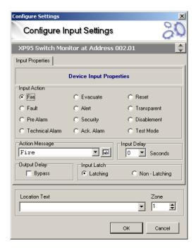
As mentioned previously, because this is fundamentally a fire system, automatic sensors cannot have their action attributes changed For sensors the attributes, which may be altered, are as follows:
