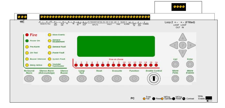
With the lid of the control open, more controls are revealed. These controls are strictly for service personnel and should not be operated by the user under any circumstances. Opening the front cover also gives access to the PC connection port for programming.
