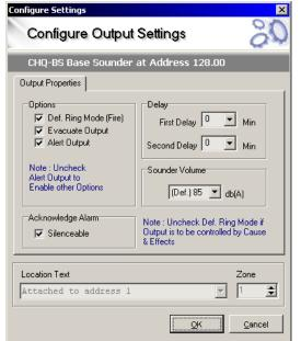
**NOTE:** If a loop sounder is controlled by a cause and effect operation, then the Tech Alarm tone will be used when the sounder is energised.
