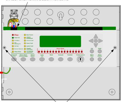
Open the outer cover using the key provided. Unplug the power terminal block from the left hand side of the circuit board, remove the two screws holding the plate in position and then remove the complete circuit board and plate.
