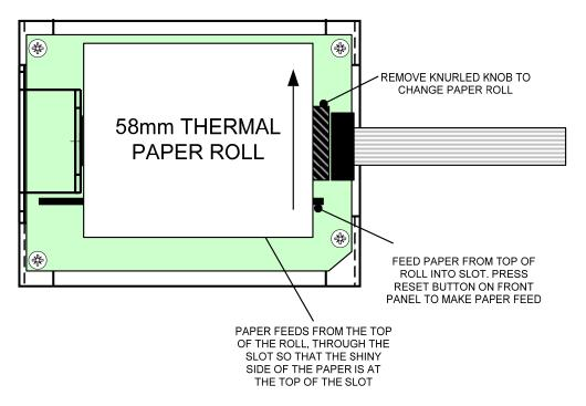
The thermal paper used in the printer is sensitive on one side only. For correct operation it is important that the paper is fed into the mechanism as per these instructions. Failure to do this will prevent correct operation of the printer.
