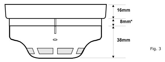
\*Shown with the YBN style of Base at 8mm, other bases such as the YBO style are deeper.
