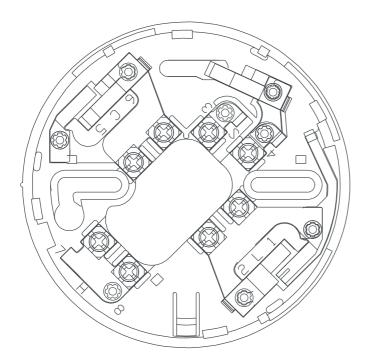
The new YBO Bases are wired exactly the same as the previous YBK style, with the exception of the YBO-R/5PA.
