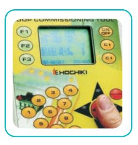
The Hochiki Loop Commissioning Tool, model TE-LCT, is a powerful yet easy to use loop installation and commissioning device. It has been designed to allow System Engineers to easily verify and test loops of Hochiki ESP devices before the control panel is installed/ commissioned.
