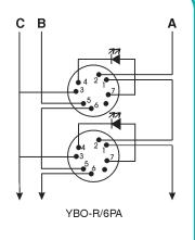
RC Relay Contacts - a flying lead on either terminal 7 or 8 selects either N/C or N/O (supplied as N/C)
