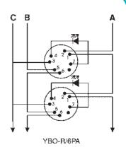
RC Relay Contacts - a flying lead on either terminal 7 or 8 selects either N/C or N/O (supplied as N/C)
