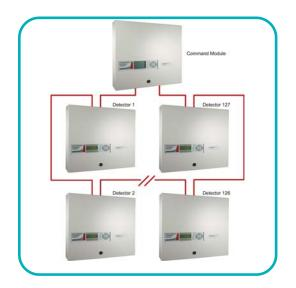
Model FIRElink-CM is a standalone Command Module designed to provide a single location display, control and interfacing option for systems of up to 127 FIRElink detectors on a network and allows global programming of all detector functions simultaneously.
