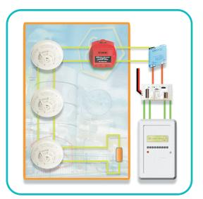
Model CHQ-Z(I.S.)/OEM is Dual Circuit Controller which is fully compatible with Hochiki's ESP analogue addressable protocol and I.S. equipment. It is supplied as an OEM version (as illustrated) which can be fitted within an IP67 rated enclosure. Addressing is achieved via simple DIL switches:
